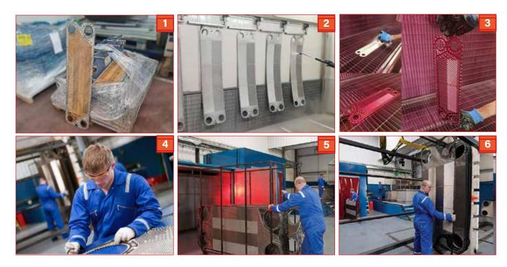
You can also return the complete plate heat exchanger, to our works for refurbishment. This service will also include a full hydraulic pressure test, complete with test certificate, before the heat exchanger is returned to site.
